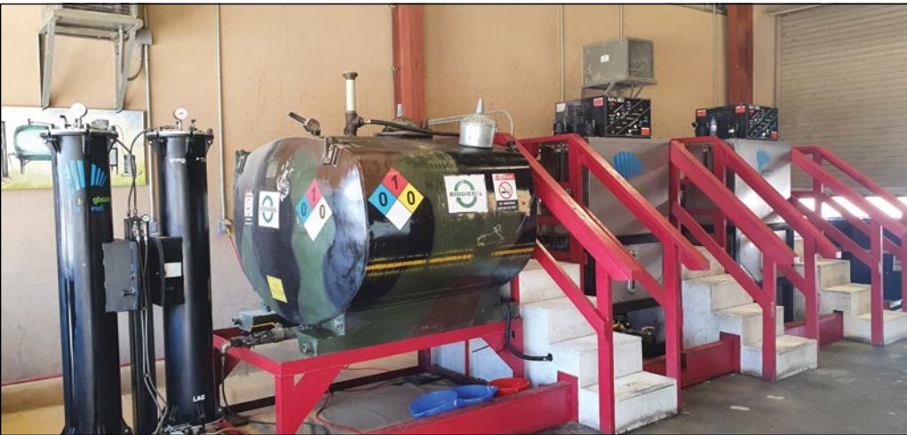
With Springboard Biodiesel equipment, Bagram Airfield in Afghanistan can process the 10,000 gallons of UCO it collects per month into fuel to power incinerators on base. PHOTO: CHRIS WAECHTER, FLUOR CORP.
